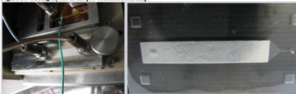
Figure 26. Tubing layout of the pre-concentration chip.
