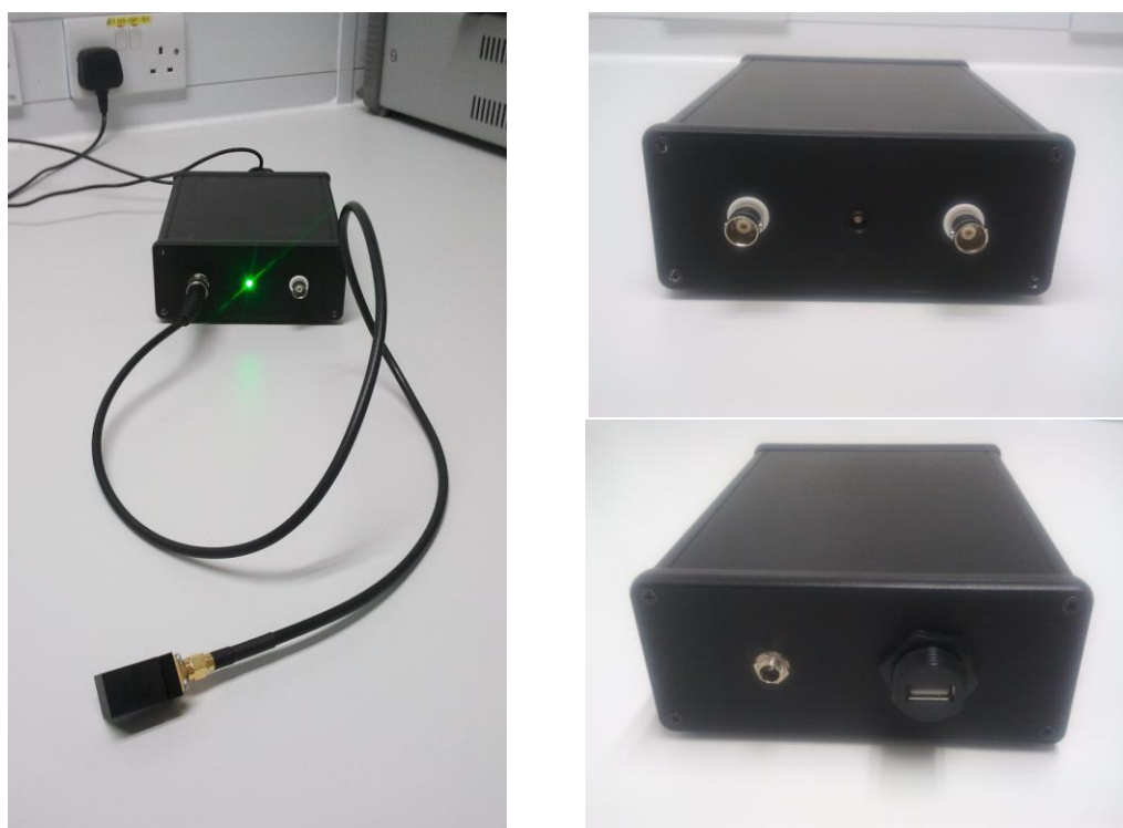
Figure 21. Radiation detector module final prototype – Radiation probe in front of the electronics box (left); electronics box front view (top right); electronic box rear view (bottom right).
