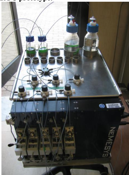
Figure 23. Pumping platform of the ROC prototype.
